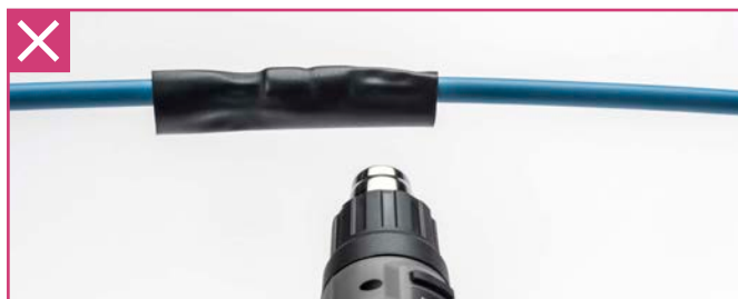
Fig. 4.16: DO NOT use heat shrink tubing for EVERLOC+ joints
