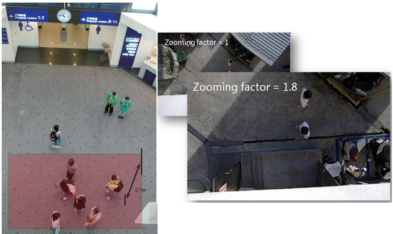
13. For Line Crossing and counting configuration, unnecessary objects should be avoided. A door, a floating curtain, and moving objects such as an escalator can cause mistakes with calculation.
