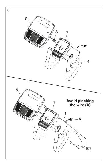
While a second person holds the Console Bracket (4) near the Frame (1), connect the wire (A) on the Console (5) to the Main Wire (115).
