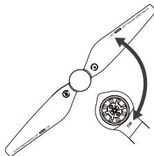
2. Press down the blade in alignment with the central axis, and rotate according to the lock marked direction by the blade lock until it is fully screwed. After installation, the propeller will pop up and lock. Removal of the blades are reverse of the above steps.
