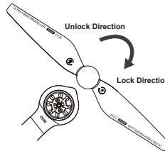
**⚠ Make sure the propellers are installed correctly and tightly.**
