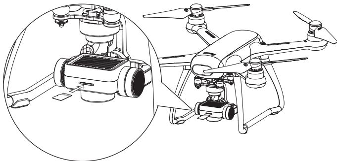
\* Insert micro SD card with the metal side up
