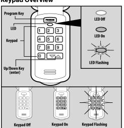
Activate keypad by opening battery compartment door to begin programming.
