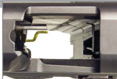
Sear Deactivation Lever for Disassembly Without Pulling the Trigger
