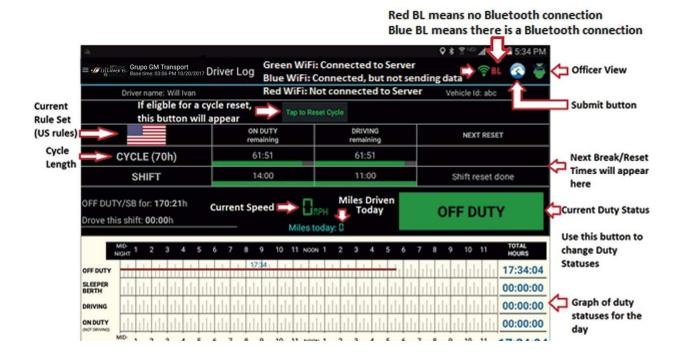
NOTE: Officer with a Green face means no diagnostic errors, Orange means at least one diagnostic error, and Red means at least one malfunction.
