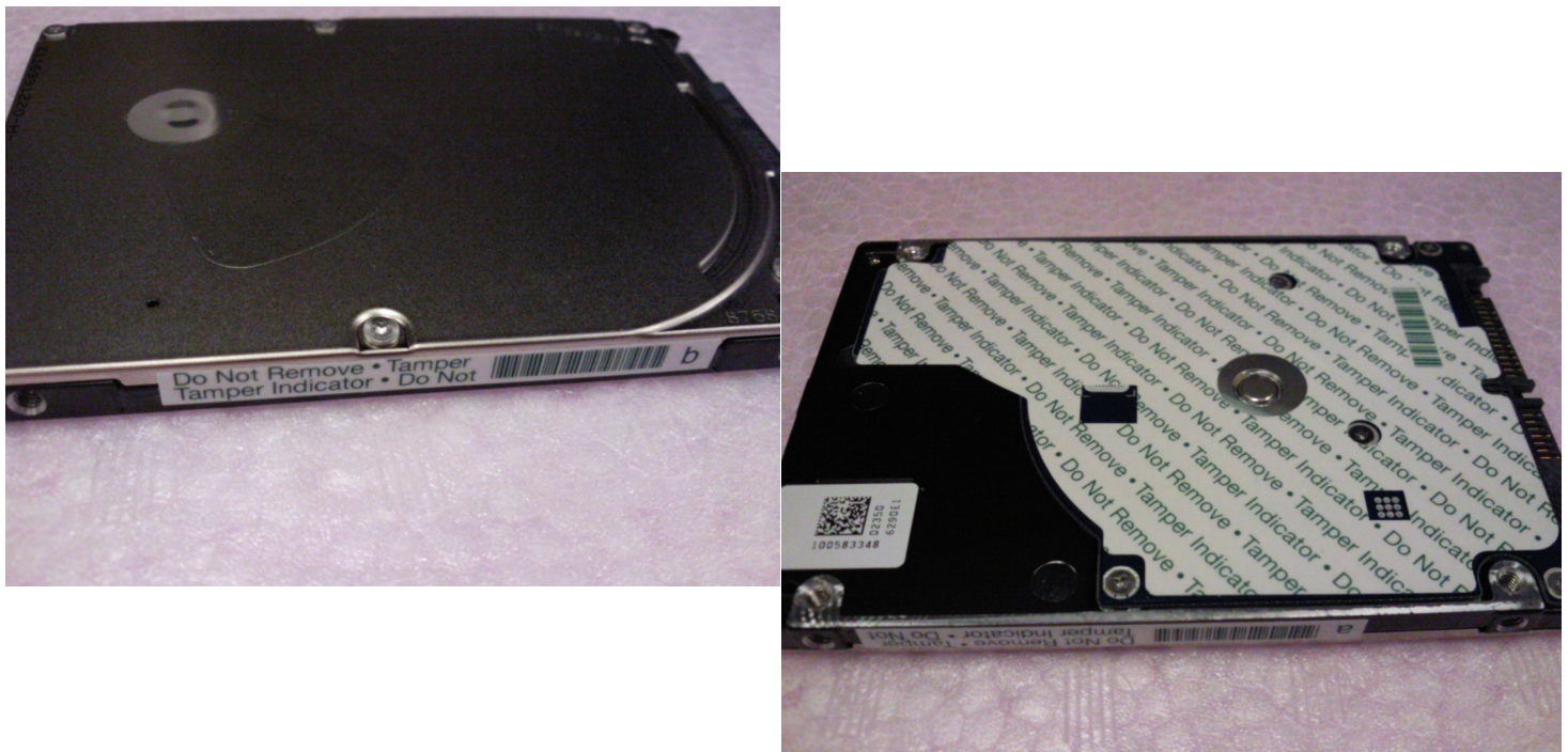
Figure 4 Example of FIPS tamper evidence labels.
