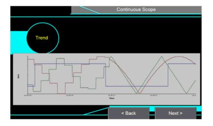
Here the first half of the trend is filled whilst the OCS was running a very processor intensive graphics screen, and at the midpoint changed to much simpler graphics display.
