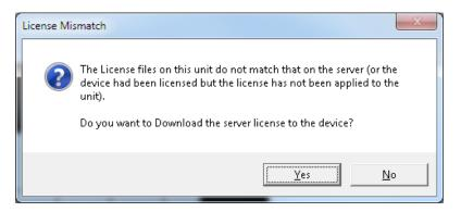
Clicking 'Yes' triggers Cscape to connect with the Horner WebMI site via internet connection. The license file is retrieved and sent to the OCS/microSD via whatever connection method is being used whether it is serial, USB, or Ethernet.
