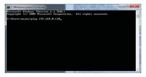
If there is a successful connection established, the command will return a response such as "Reply from 192.168.0.110: bytes=32 time=1ms TLL=64".
