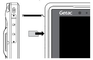
3. Close the cover and tighten the screw.
