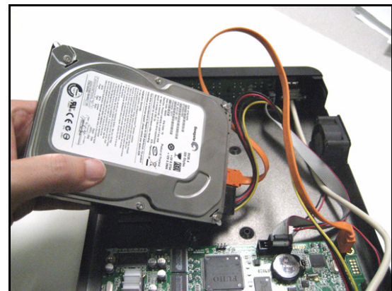
Figure 21.3 Carefully remove the HDD from housing.
