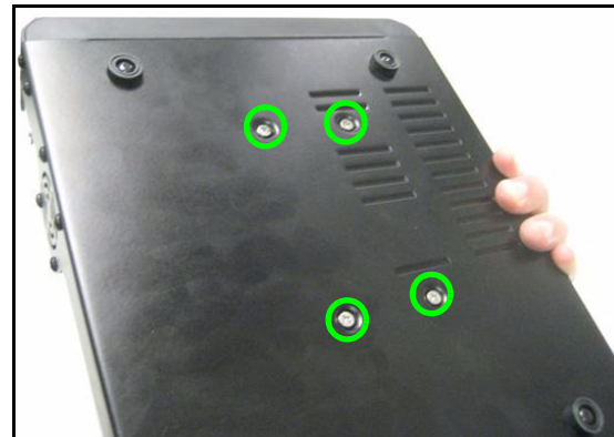
Figure 21.2 Support the HDD with your hand and remove mounting screws.
