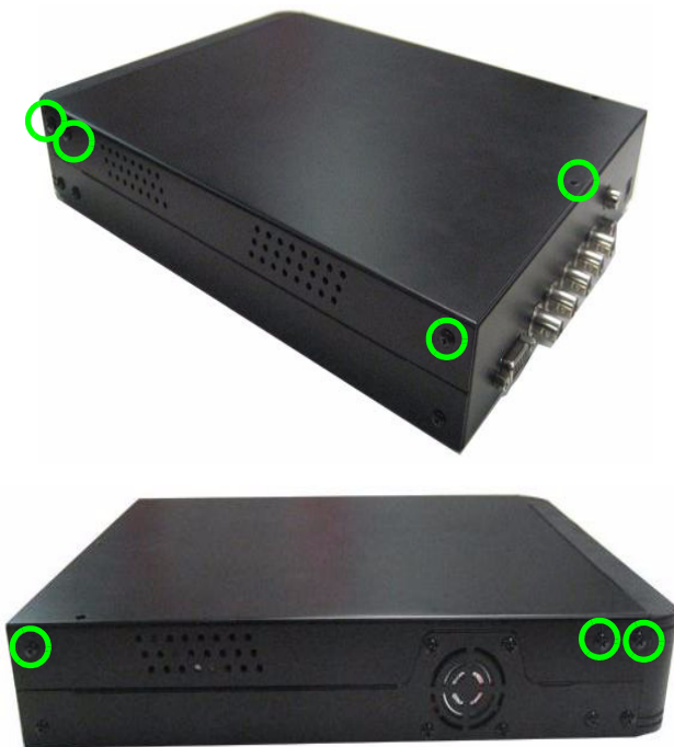
Figure 21.0 Remove seven screws from cover
