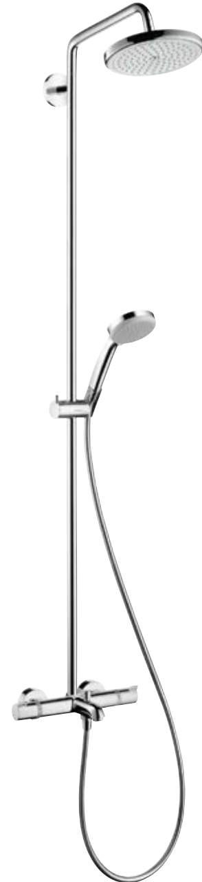
Croma® 220 Air 1jet Showerpipe for bathtub with swivelling Croma 220 Air 1jet overhead shower (17 l/min), Croma 100 Vario hand shower (15 l/min), Ecostat Comfort bath thermostat (20 l/min), shower arm 400 mm # 27223, -000 Height of the Showerpipe can be reduced
