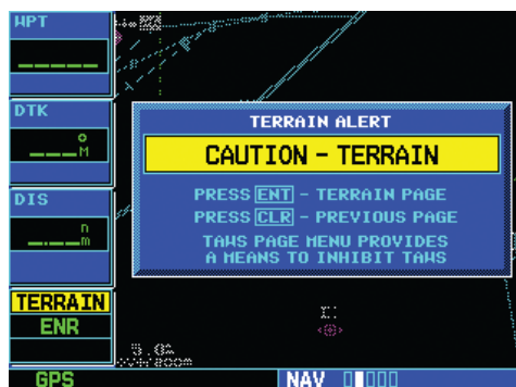
Figure 11-3 Caution Alert Pop-up
