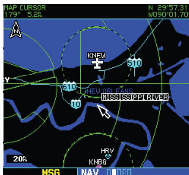
Figure 6-39 Activate Panning Function
