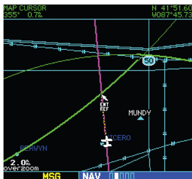
Figure 2-22 Using Pointer to Measure Distance and Bearing
