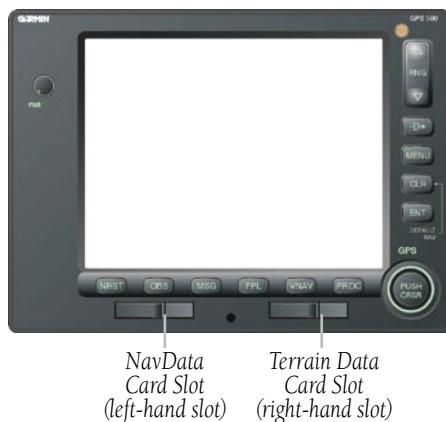
Figure A-1 Data Card Slot Locations
