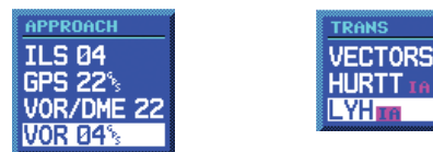
Figure 5-11 Approach and Transitions Windows
