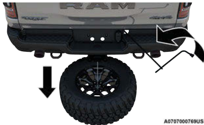
Pulling The Spare Tire Out
