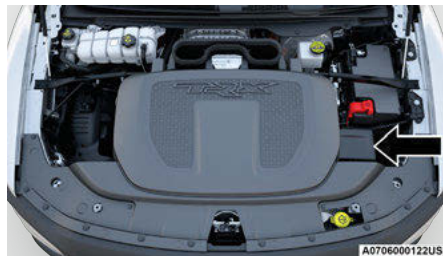
Power Distribution Center
