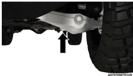
Front Lifting Point
