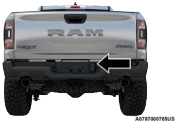
Access Hole Cover Location
