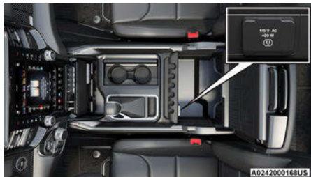
Center Console Power Inverter Outlet
