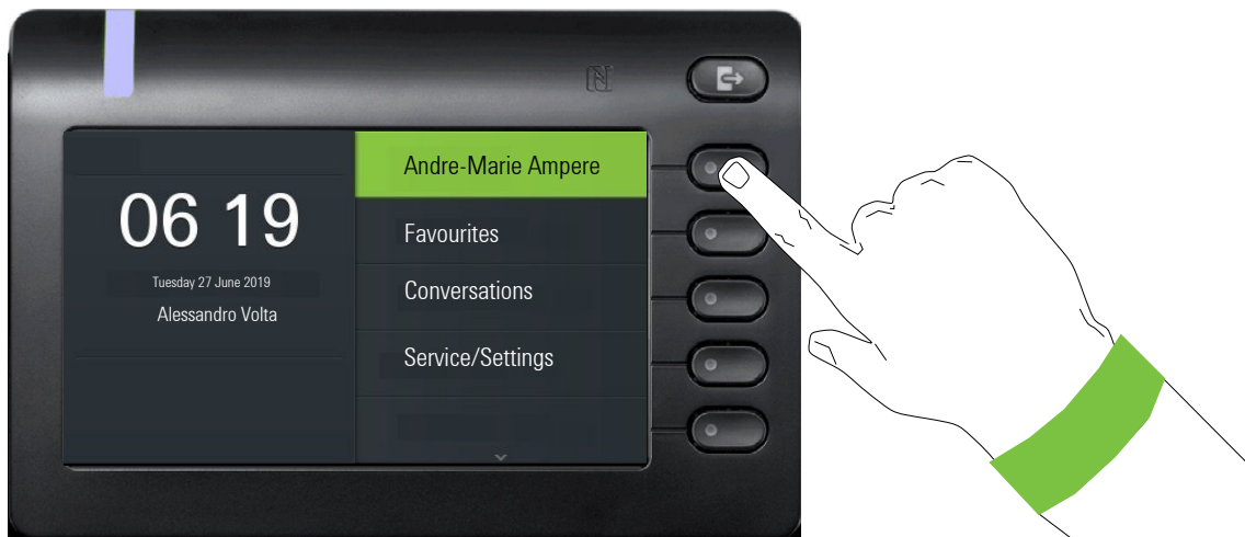
Selecting the first softkey will take you back to the previous display.
