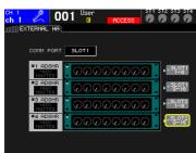
Using the PORT SELECT buttons, select the input ports to which the external HA (SB168-ES) is connected in groups of 8 channels.
