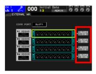
7. Open the Rack page and go to the External HA screen. Use the External HA Port Select button to assign all the displayed HA controllers to the slots. (This setup is not part of SCENE MEMORY and is set for all SCENEs.)
