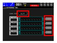
In the EXTERNAL HA screen, move the cursor to the COMM PORT box, use the dial or the [DEC]/[INC] keys to select "SLOT1", and press the [ENTER] key.
