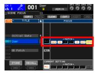
9. In the SCENE requiring the SB168 patch, change focus from [ALL] to [RACK] [HA] .... [IN] [OUT] [With Send].
