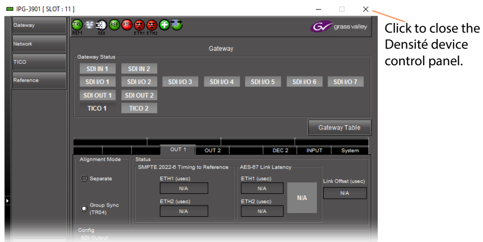
Fig. 2-18: Example Densité Device Control Panel
