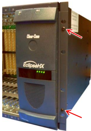
Figure 2-5: Attaching the Eclipse HX door to the matrix
