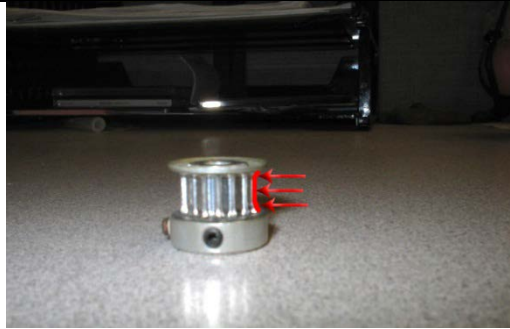
Worn pulley Figure 12
