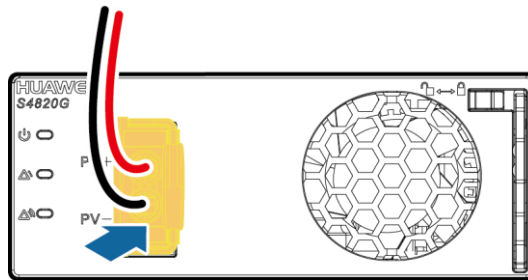
Figure 6-22 Reconnecting the solar input cable to the new SSU
