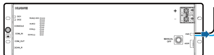
Figure 6-41 Removing the ESM power cable terminal
