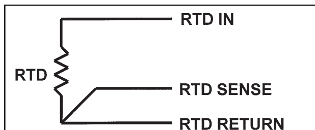
FIGURE 15-4. Three-Wire RTD Configuration.
