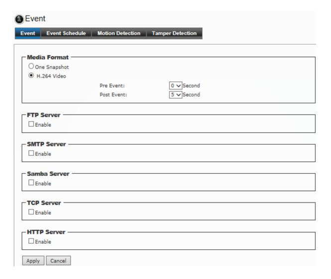
Media Format: Select One Snapshot to send the alarm message with one still image captured by the camera, or select H264 Video to send the alarm message with one video clip recorded by the camera.
