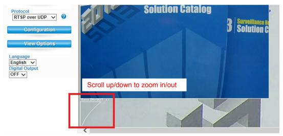
Note: Digital zoom uses computer algorithm to enlarge the video and may lose some details.
