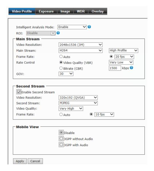
Intelligent Analysis Mode: You can select Enable or Disable to switch the IVS function.
