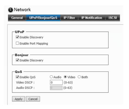
UPnP: The camera supports UPnP (Universal Plug and Play), which is a set of computer network protocols that enable the device-to-device interoperability. Select the Enable Discovery option to enable the feature.
