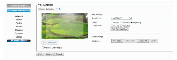
Select Sensitivity to set the detection sensitivity level. Higher sensitivity will make it easier to detect and less objects missing, but more misjudgments.
