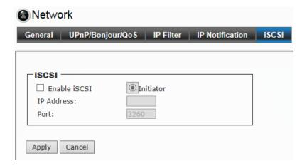
Enable the iSCSI and key-in server IP address and Port number. The disk of the server will be the storage in IP camera setting.
