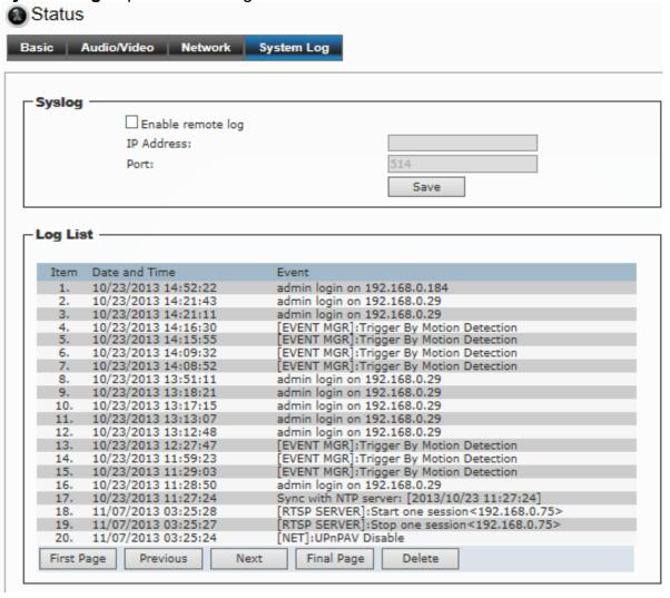
• **Enable remote log:** Enter the IP address to enable the remote log function.
