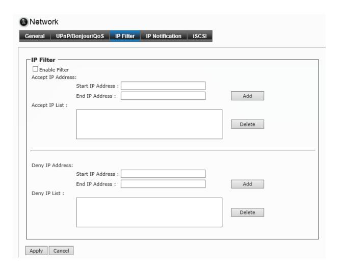
The IP Filter allows the administrator of the camera to restrict the users within a certain range of IP addresses to access into the camera. Select the **Enable Filter** option and assign the range of IP addresses that are allowed to access into the camera in the **Accept IP Address** field; or assign the range of IP addresses that are blocked to access into the camera in the **Deny IP Address** field.
