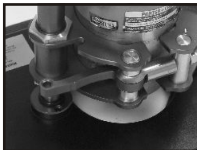
CLAMP OPEN The cam lock design spreads the clamp when fully opened.
