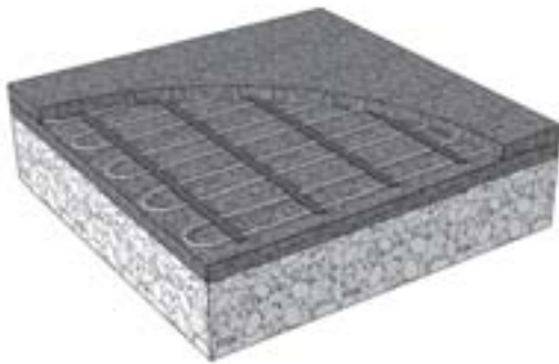
ProMelt embedded in asphalt
