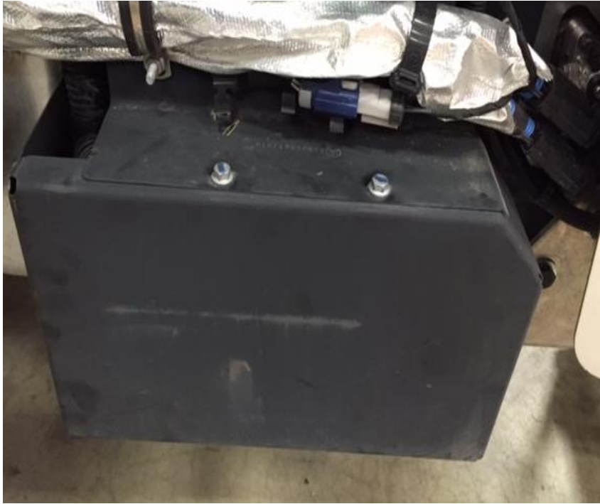
Figure 14 – ACM Cover Installation
