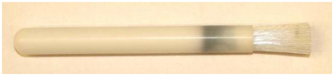
Figure 10 – Insulative Nylon Brush used for Connector Cleaning
