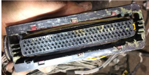
Figure 8 – ATS Harness 21-pin and 120-pin Connector Inspection
