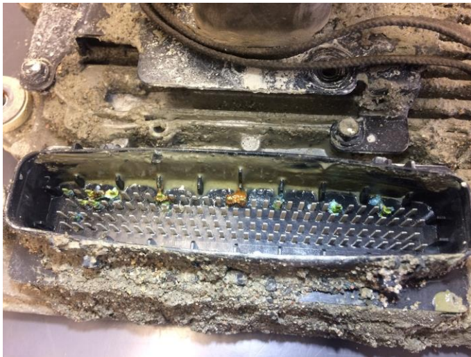
Figure 9 – ACM 21-pin and 120-pin Connector Inspection
