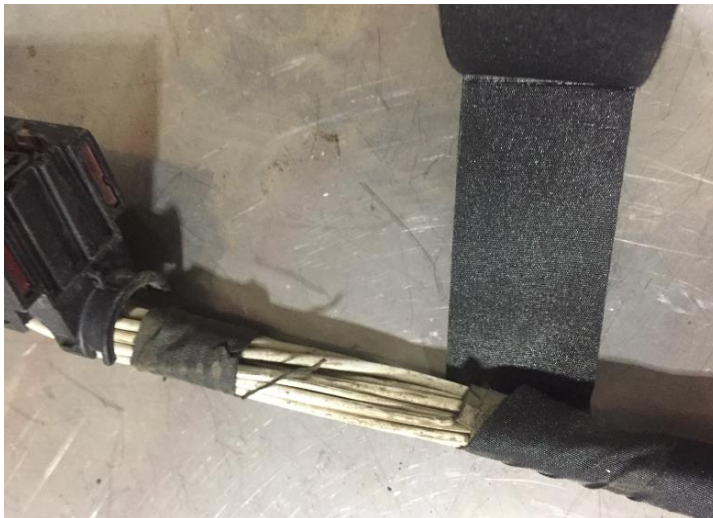
Figure 11 – Anti-Chaffing Tape Installation
