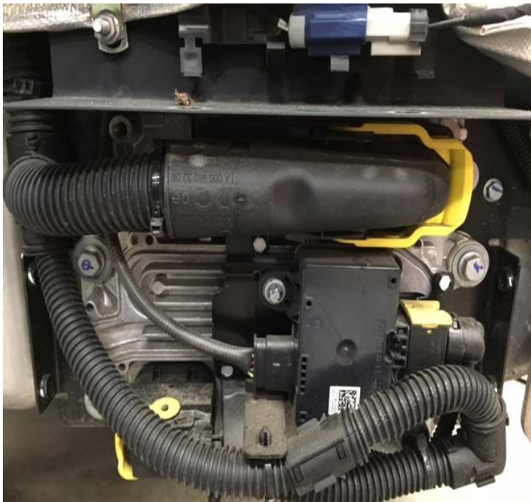
Figure 3 – Harness Routing and Zip Tie Location
