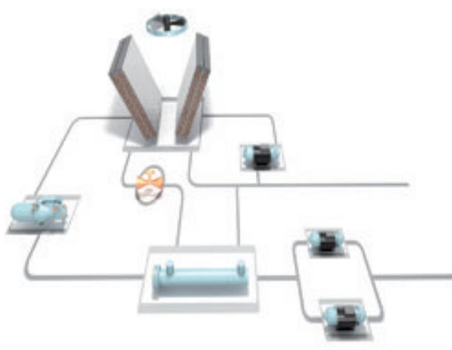
Free-cooling is an efficient method to reduce energy consumption at low outside air temperatures. It enhances energy optimization in data center and process cooling.
