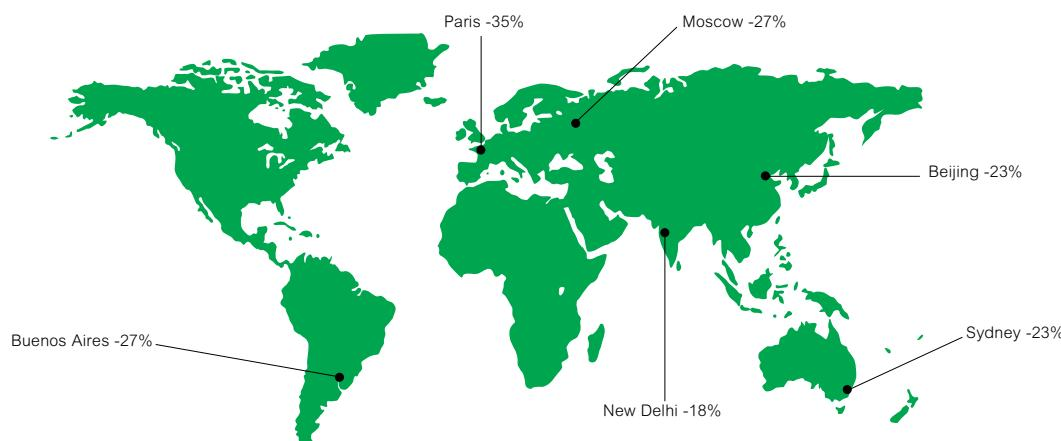
Data comparing traditional free-cooling units at 18/24°C water temperature with free-cooling adiabatic chillers at 18/28°C water temperatures.
