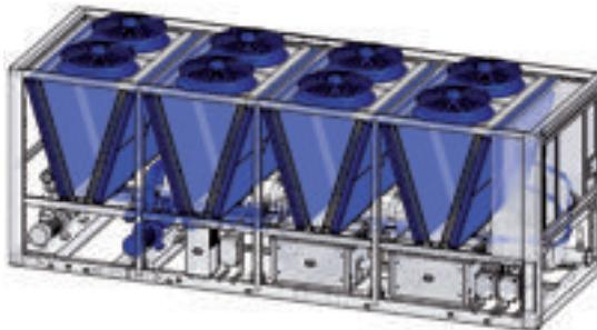
Aquaflair chillers are designed to integrate the main electrical and hydraulic components onboard the units. Free-cooling circuit, primary pumps, VSDs, water tanks, and automatic transfer switches are available to be factory installed which reduces the design and installation phases and allows a solution ready to be used.
