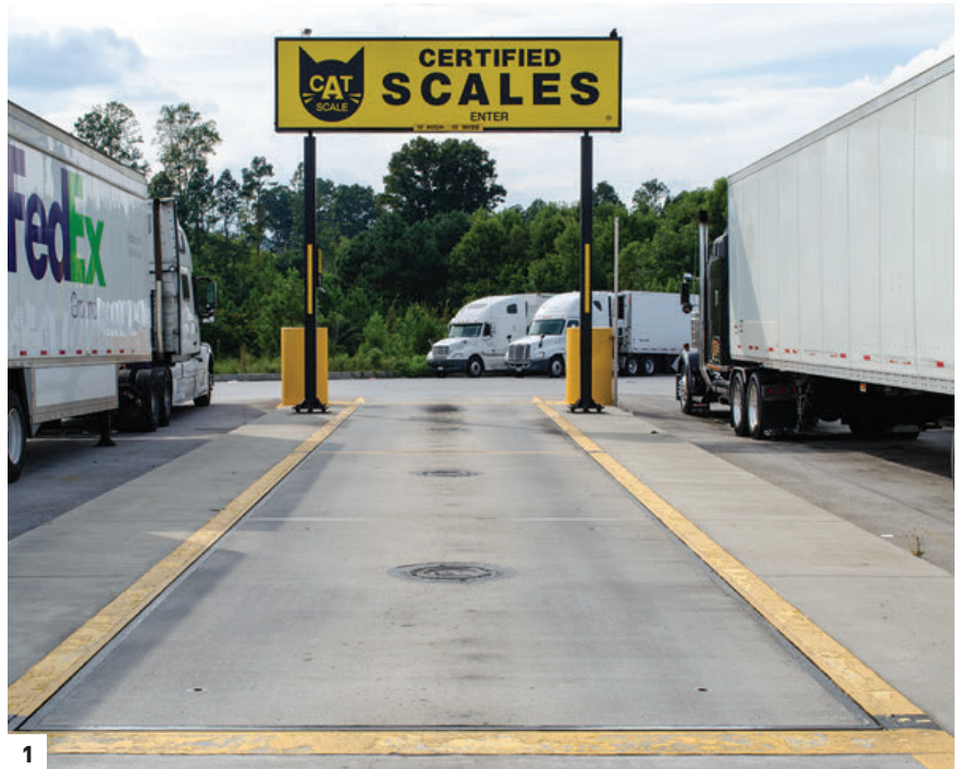
[1] Approaching the scale, you should be able to see the lines or segments on the scale pavement as well as the yellow boundary that indicates the area that is outside the weighing area. This allows you to position the coach with the steer tires and rear tires on different sections of the scale. Notice how this scale has a wide area outside the yellow line (apron) that is level with the scale.
