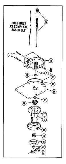
**STEP 6:** Install plastic plug in top of housing, re-engage elevating gear in worm gear, replace pin and retaining ring.
