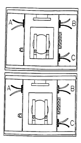
When you have the optional 50 amp service, the red wire shown on the following diagram will be providing power to the rear air conditioner whether you are plugged into city power or operating the generator.
