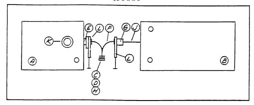
A. 601493 Black Tank B. 601492 Grey Tank Bayonet Ring 0 C. 601251 Bayonet Cap D. 601250 E. 601432 Adapter 3 Way Elbow F. 600866 3" Coupler G. 600289 3" Dia x 3" H. 601160-04 3" Dia x 10" J. 601160-04 K. 601266 4 x 3 Closet Flange L 601430 3" Gate Valve
