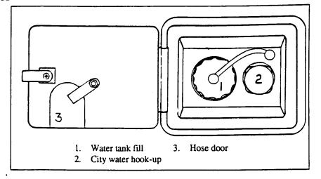
have a spare hose should one fail or become damaged unexpectedly. Turn the water heater bypass to the normal flow position as described under self- contained.
