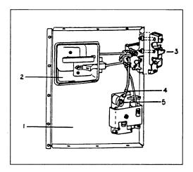
Access to the linkage mechanism of the lock is gained by removing the two screws holding the lock handle and the center panel of the inside door skin. This will expose the door lock assembly, as shown in the illustration.
