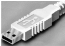
Figure 5-3 -- Host connector end of USB cable.
