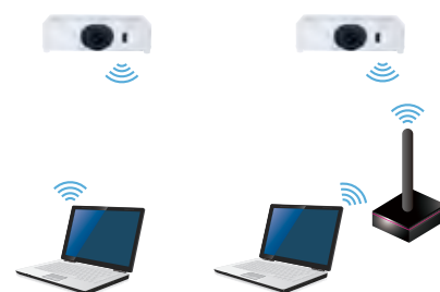
Without an access point
