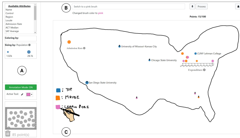
Fig. 3. The system's interface as Sarah concludes her exploration: (A) Side panel with (from top to bottom) the attribute summary container, legends for global coloring and sizing attributes, annotation options, and a virtual bin for filtered points; (B) Speech input and feedback row; (C) Main canvas. Here, Sarah is using the brush tool to draw a custom color legend.
