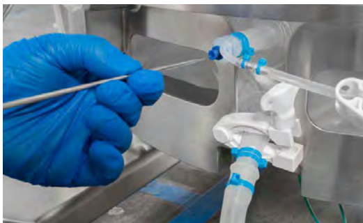
Figure 3.26. Inserting the RTD into the thermowell.
