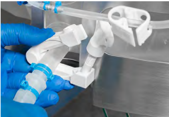
Figure 3.25. Closing bar clamp on drain line.
