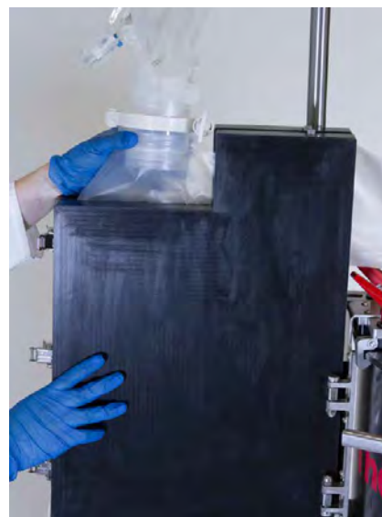
Figure 3.40. Closing the condenser door.
