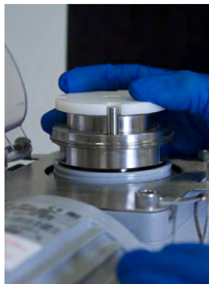
Figure 3.21. Aligning the motor drive keyway.
