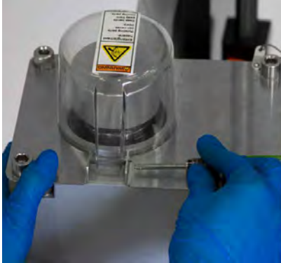
Figure 3.48. Removing the latch pin.
