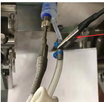
Figure 3.14. Media ground clip connection.
