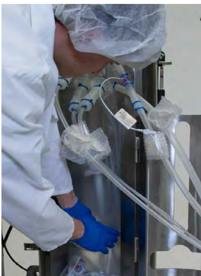
Figure 3.13. Aligning the connector ports and probes.
