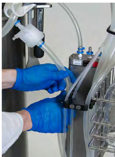
Figure 3.9. Line setup on the cable management system.
