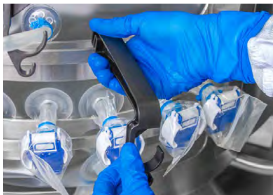
Figure 3.80. Attaching a probe clip.
