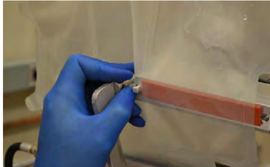
Figure 3.15. Positioning the BPC cutout over the alignment pin in a pinch clamp.
