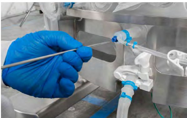
Figure 3.61. Inserting a sensor into the thermowell.
