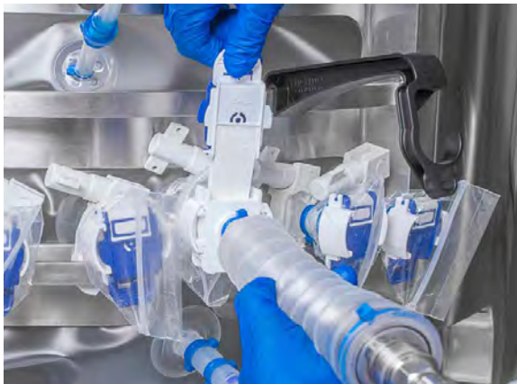
Figure 3.79. Pulling tabs to remove the paper membranes.
