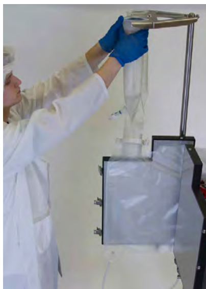
Figure 3.39. Exhaust filter and condenser setup.
