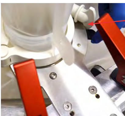
Figure 3.36. Locking the exhaust port.
