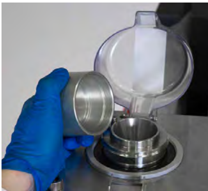
Figure 3.50. Removing the drive shaft cap.
