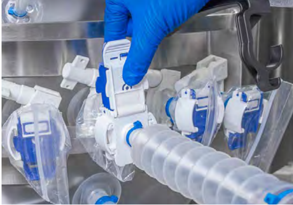
Figure 3.78. Squeezing connectors together.
