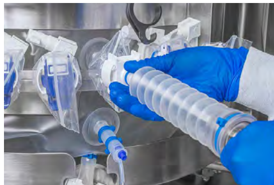
Figure 3.81. Installing the pre-sterilized sensor.
