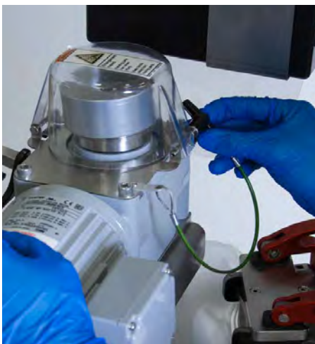
Figure 3.19. Removing the latch pin from the motor assembly.
