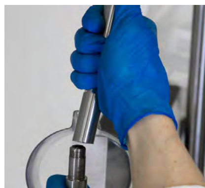
Figure 3.54. Connecting the upper drive shaft segment.
