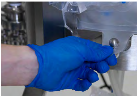
Figure 3.12. Aligning a hanging tab with the pin.
