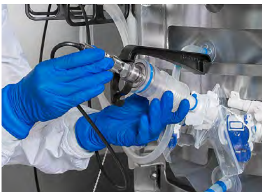
Figure 3.83. Lifting the probe upward into the spring.
