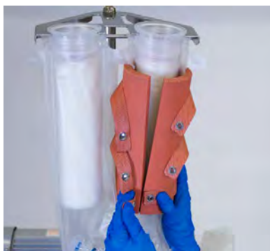
Figure 3.68. Snapping a vent filter heater onto the filter.
