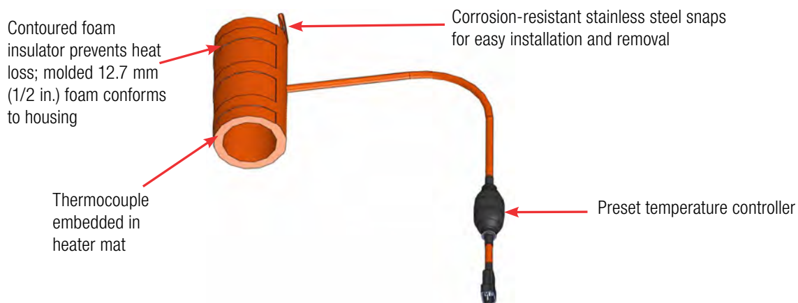
Figure 4.18. Vent filter heater.
