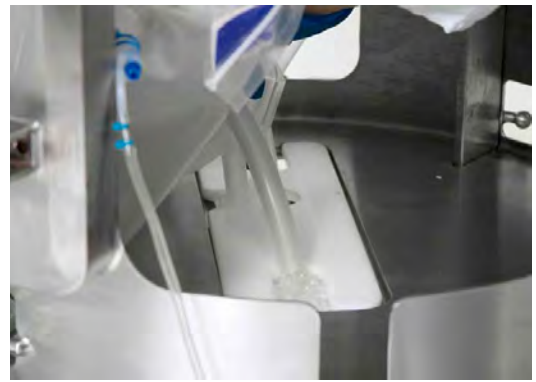
Figure 3.42. Replacing the guide plate.
