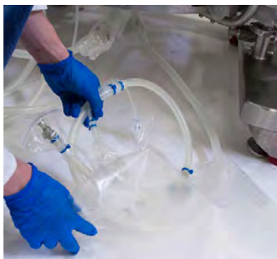
Figure 3.59. Removing the drain line set from a polybag.
