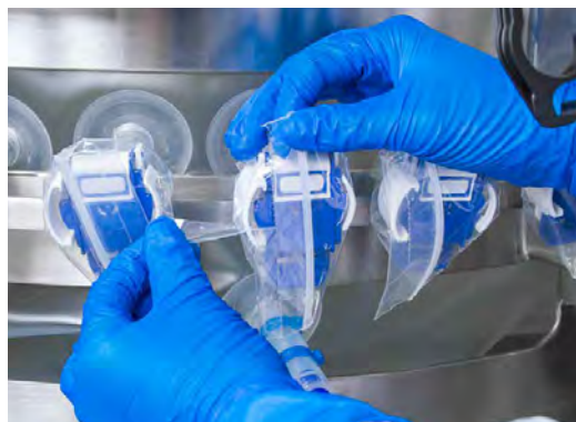
Figure 3.74. Pulling the tear strip.
