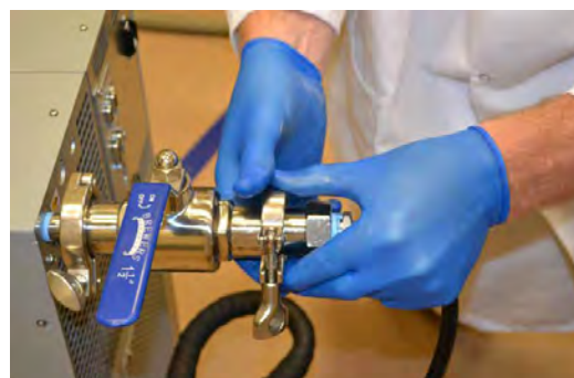
Figure 2.9. Attaching a clamp to a line.
