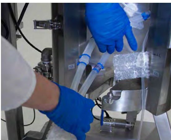
Figure 3.5. Routing the sparge and bottom drain lines.
