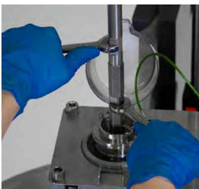
Figure 3.53. Tightening the drive shaft connections.
