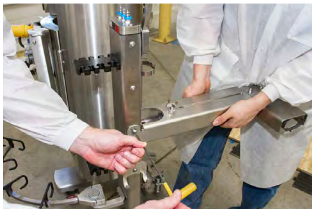
Figure 2.14. Attaching arm to cable management system.
