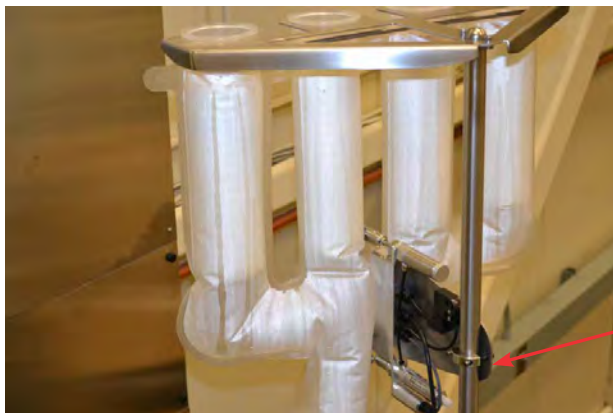
Figure 2.13. Pinch clamp installed on a 300 L S.U.F.
