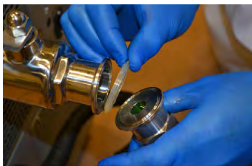
Figure 2.8. Attaching line to a TCU unit.
