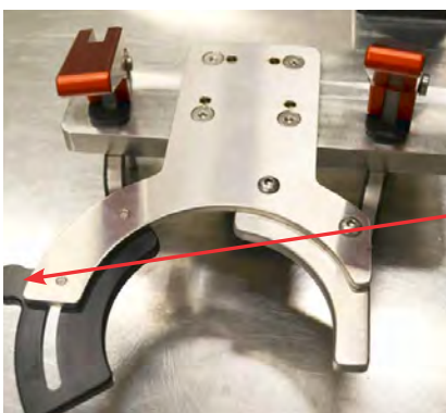
Figure 3.35. Exhaust port sliding latch (removed from the tank).
