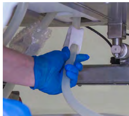
Figure 3.60. Placing a clamp on the drain line.
