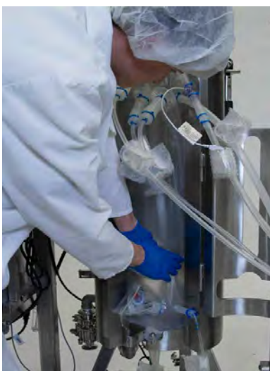
Figure 3.4. Routing the bottom ports through the bottom of the outer support container.
