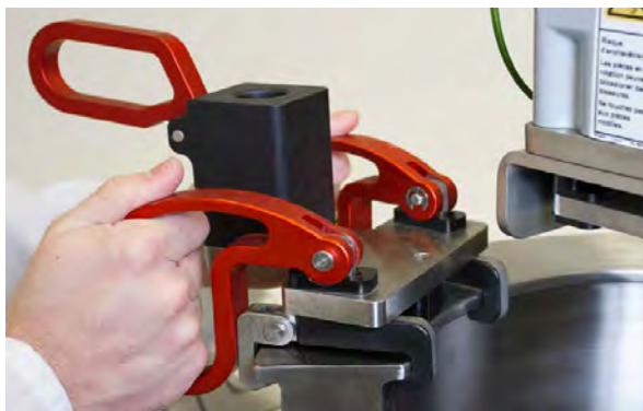
Figure 2.5. Clamping the exhaust filter bracket to 30 L S.U.F. tank.
