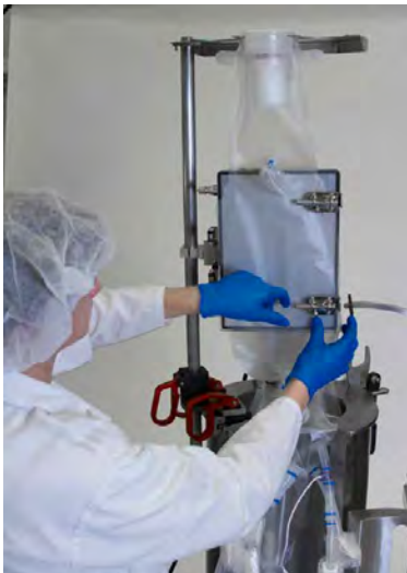
Figure 3.7. Loading of an optional condenser bag.
