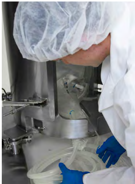
Figure 3.43. Sparge and drain line extension.
