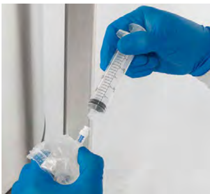
Figure 3.107. Connecting the syringe.
