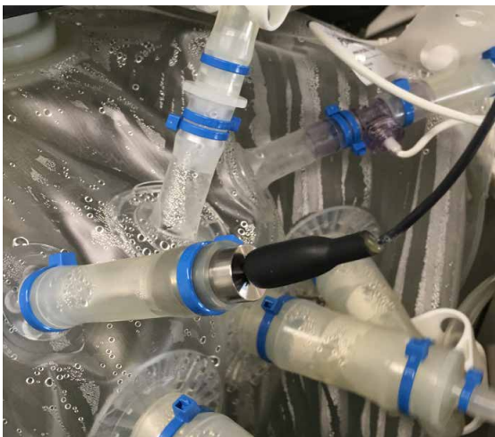
Figure 3.62. Foam sensor wire connected in port.
