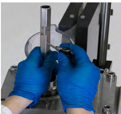
Figure 3.51. Inserting the lower section and securing it with a latch pin.
