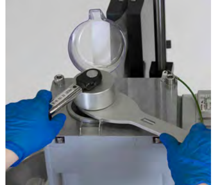
Figure 3.49. Opening the drive shaft cap.
