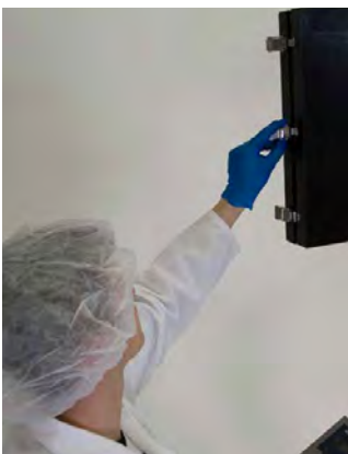
Figure 3.65. Opening the condenser door (300 L S.U.F. unit).
