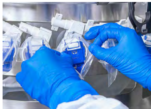
Figure 3.75. Removing the plastic covering from the connector.
