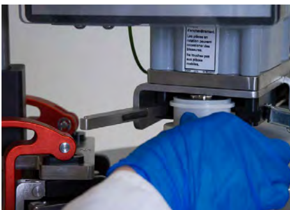
Figure 3.3. Inserting the bearing port.
