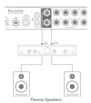
All the line output connectors are 3-pole (TRS) ¼" (6.35 mm) jack sockets, and are electronically balanced. Typical consumer (hi-fi) amplifiers will probably have unbalanced inputs, either on phono (RCA) sockets, or via a 3.5 mm 3-pole jack plug intended for direct connection to a computer. In either case, use a suitable connecting cable with jack plugs at one end.
