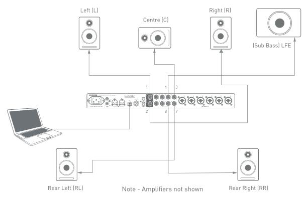
The table below summarises how some common multichannel formats could be mapped to the Scarlett 18i20's outputs for monitoring purposes, as configured within the DAW:
