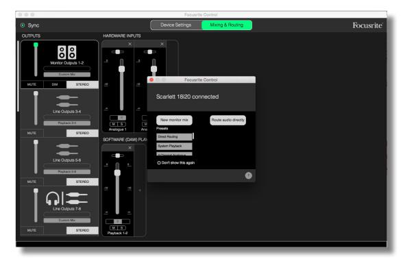
The following table provides the channel routings when preset option "Direct Routing" is selected in Focusrite Control; see the screen image on page 18. Note that as the channel count available via the ADAT optical ports is reduced at higher sample rates, the default routings change slightly at the higher rates.
