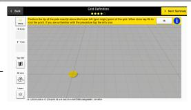
Make sure that RTK has been fully established beforehand. Otherwise this step cannot be completed successfully.
