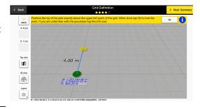
Adhering to the grid size limits (minimum 4 x 4 m / 12 x 12 ft, maximum 11 x 11 m / 33 x 33 ft) at 50 cm / 1.5 ft intervals and the establishment of full RTK ensures that this step is completed successfully.
