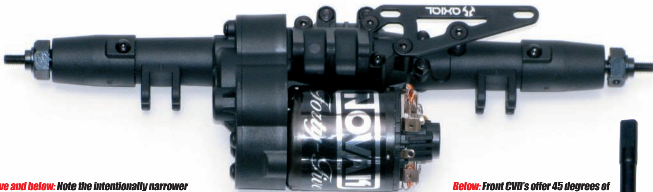
Above and below: Note the intentionally narrower rear axle to help clear gates in use
