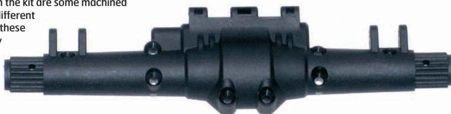
Above: The straight through rear axle and metal spool Below: Years of Axial's development and knowledge rolled into just one rig..
