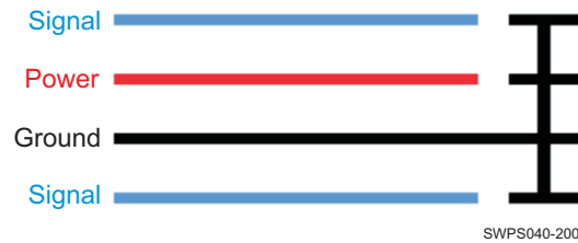
Figure 8-19. Guard Ring Routing
