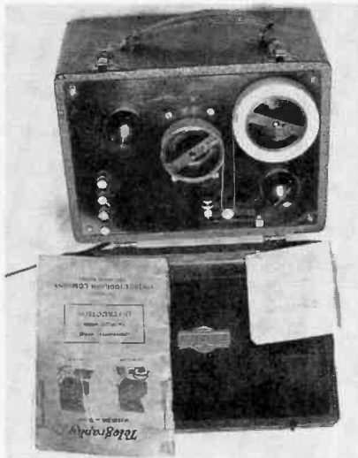
An Instructograph AC-powered code-practice machine. This model had a built-in oscillator. The knobs were used to control volume and speed.
