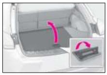
**3** Unhook the string on the backside of the deck board.
