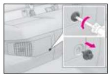
3 Remove the air intake vent cover.
