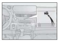
The security indicator flashes after the power switch has been turned off to indicate that the system is operating. The indicator light stops flashing after the power switch has been turned to ACC or ON to indicate that the system has been canceled.
