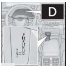
While the power switch is in the brake pedal depressed, shift the shift lever while pushing the shift release button on the shift knob.
