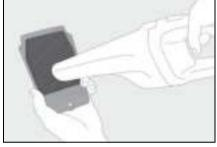
6 Reinstall the filter to the cover.
