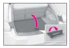
2 Unhook the string on the backside of the deck board.
