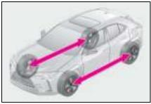
To equalize tire wear and extend tire life. Lexus recommends that tire rotation is carried out at the same interval as tire inspec-
