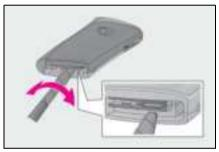
3 Remove the depleted battery using the small flathead screwdriver.
