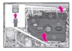
5 Connect a positive jumper cable clamp to A on your vehicle and connect the clamp on the other end of the positive cable to B on the second vehicle. Then, connect a negative cable clamp to C on the second vehicle and connect the clamp at the other end of the negative cable to D.
