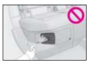
When cleaning the air intake vent, make sure to only use a vacuum to suck out dust and clogs. If a compressed air blow gun, etc. is used to blow out dust and clogs, the dust or clogs may be pushed into the air intake vent, which may affect the performance of the hybrid battery (traction battery) and cause a malfunction
