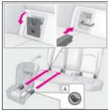
3 If the child restraint has a top tether strap, follow the child restraint manufacturer's operation manual regarding the installation, using the top tether strap to latch onto the top tether strap anchor. (→P.54)
