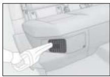
Remove the dust from the air intake vent with a vacuum cleaner etc.
