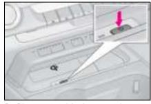
Place a portable device on the charging area with its charging surface facing down.
