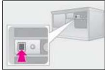
3 Press and hold the desired HomeLink<sup>®</sup> button (inside the vehicle) for 2 seconds and release it. Repeat this sequence (press/hold/release) up to 3 times to complete programming. If the garage door opener motor operates when the HomeLink button is pressed, the garage door opener motor recognizes the HomeLink signal.
