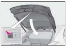
Close the back door and lock all doors (close & lock function)
