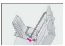
3 Fully extend the shoulder belt and allow it to retract to put it in lock
