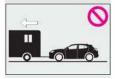
AWD models: Never tow this vehicle with any of the wheels on the ground. This may cause serious damage to the hybrid transmission and AWD system.
