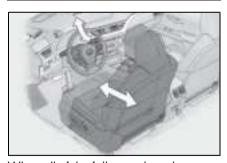
When all of the following have been performed, the driver's seat and steering wheel are automatically adjusted to a position that allows driver to enter and exit the vehicle easily.
