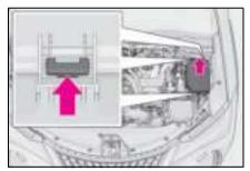
► Engine compartment: type B fuse box
