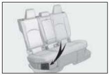
There is an air intake vent under the right side of the rear seat for the purpose of cooling the hybrid battery (traction battery). If the vent becomes blocked, the hybrid battery (traction battery) may overheat, leading to a
