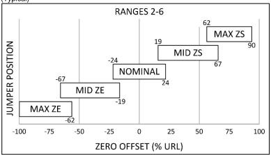
% Zero Offset values and jumper positions indicated are approximations. Select jumper position as needed to achieve the desired calibration.
