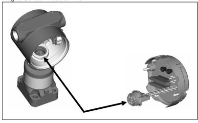
Figure 5-10 – Installation of Electronics Assembly Connector Plug
