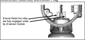
Push the electronics assembly (4) into the electronics housing (5) and fasten with the two 6-32 captive screws. Torque each captive screw to 7in-lbs ±1 inlbs (0.8 N-m ±0.1 N-m), or hand-tight (see Figure 5-11).
