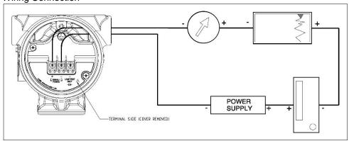
The power supply versus load limit relationship is shown in **Figure 2-4**. See qualification reports for additional details. The loop load is the sum of the resistance of the signal leads and the load resistance of the receivers. Any power supply ripple appears in the output signal.
