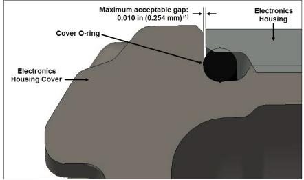
(1) If the gap exceeds acceptable limit, it will be possible to insert a 0.010 inch gap gauge at least 0.100 in (2.54 mm).
