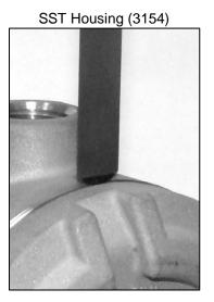
Figure 2-11b – Unacceptable Gap Between Cover and Housing
