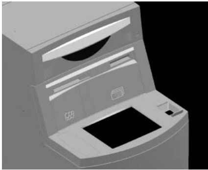
Figure 3 ATM with small palm vein pattern authentication sensor unit (CG design image).
