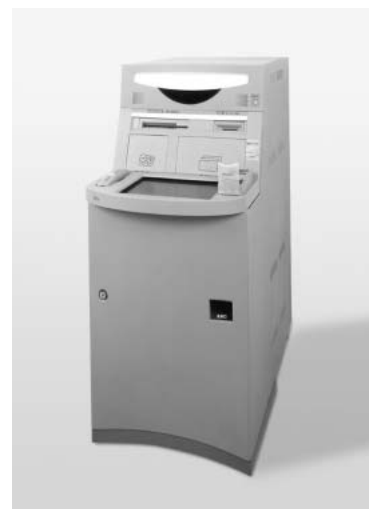
Figure 2 ATM with palm vein pattern authentication sensor unit.
