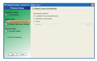
The Protocol Setup window displays lane and band detection options:
