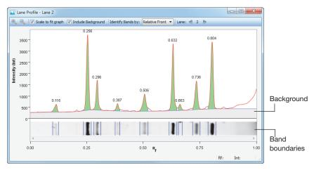
The Lane Profile option shows a cross-section view of a single lane rotated 90°.
