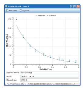
The Standard Curve dialog box displays the best curve fit for the defined standards and the bands relative to this curve for the lane selected in the image. The tabs at the bottom of the dialog box display the standard curves for three different analyses.
