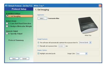
The three major processes are listed in the left pane. Numbered major steps in each process appear under these headings. To select options under a protocol step, select the accompanying checkbox. Options appear in the right side of the window. To disable any step, clear its checkbox.
