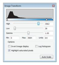
The minimum to maximum range varies depending on the light and dark values present in the image. These adjustments do not change the data. They change only the way the data are displayed. The human eye cannot see as great a range as the image contains.
