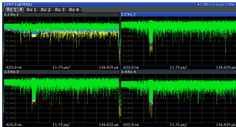
Figure 3-20: PVT Full PPDU result display for IEEE 802.11n MIMO measurements
