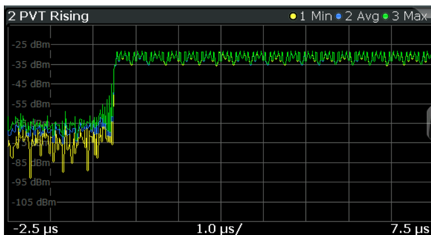
Figure 3-22: PVT Rising Edge result display
