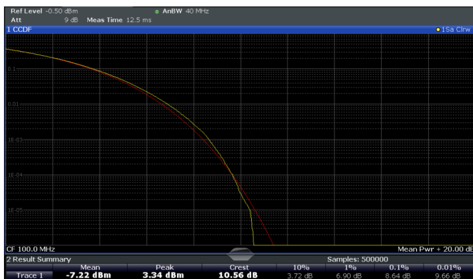
Figure 3-30: CCDF measurement results
