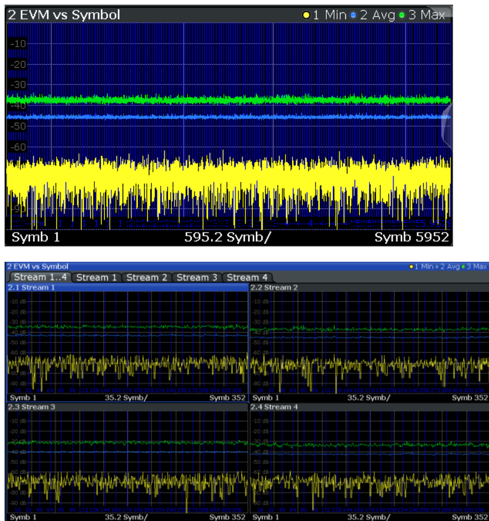
Figure 3-13: EVM vs symbol result display for IEEE 802.11n MIMO measurements
