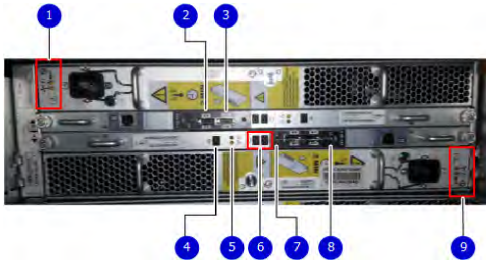
Figure 178 Back panel: Power modules and controllers
