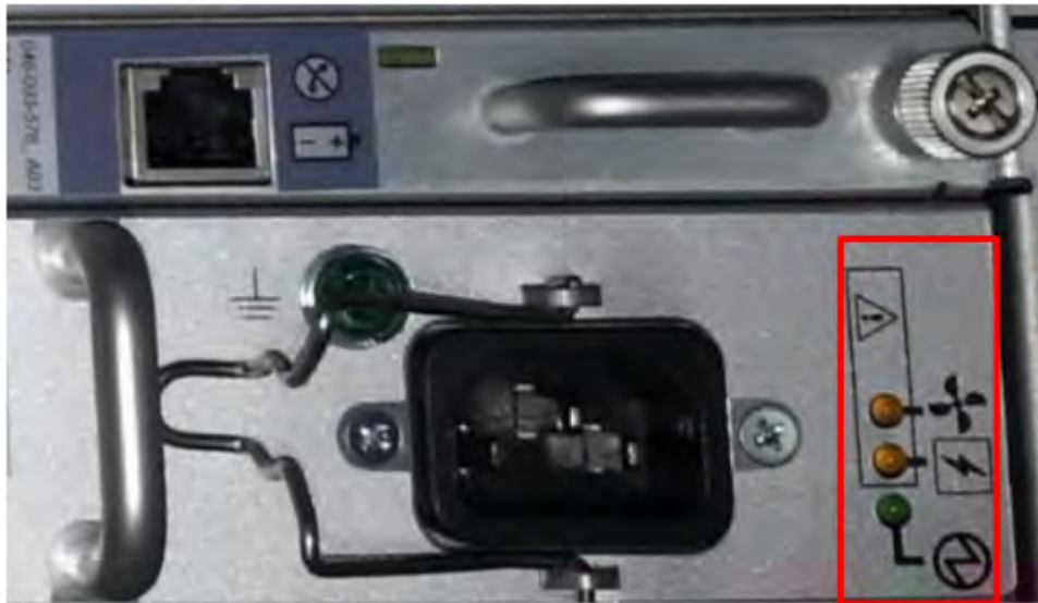
Figure 179 Power Supply A LEDs
