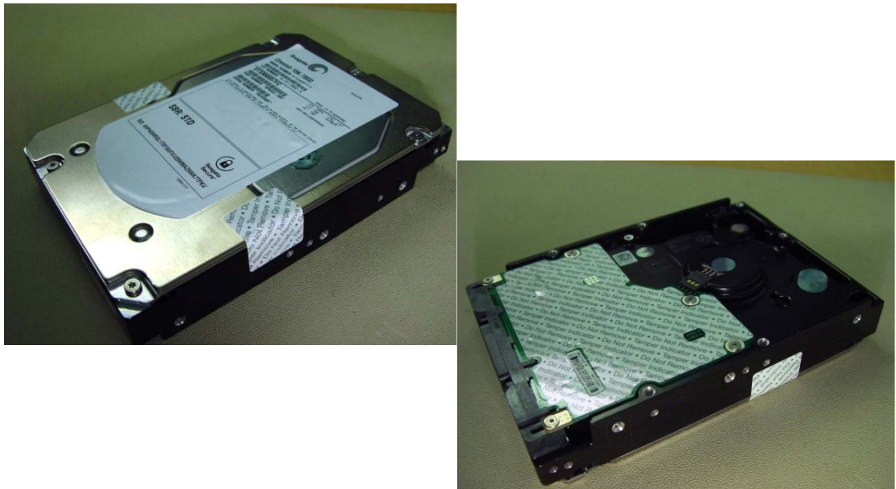
Figure 10. Example of FIPS tamper evidence labels.
