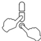
**To reset the thermostat,** press both **Down** and **Select** buttons and hold. After 3 seconds, **RST** appears. After the next 5 seconds, when **RST** disappears, release the buttons. Except for the time and date, the thermostat has now returned to its default settings.
