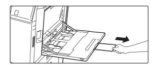
When loading paper larger than 8-1/2" x 11"R or A4R, pull out the extension guide.
