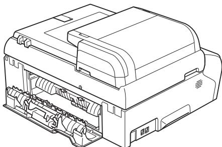
6 Using both hands, use the finger holds on both sides of the machine to lift the scanner cover (1) until it locks securely in the open position. Make sure that there is no jammed paper left inside the machine under the plastic covers. Check both ends of the print carriage.
