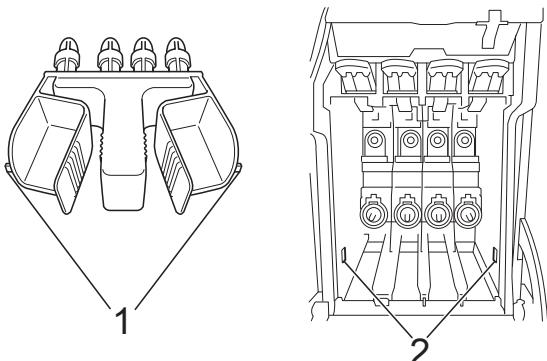
If you are not able to find the green protective part, DO NOT remove the ink cartridges before shipping. It is essential that the machine be shipped with either the green protective part or the ink cartridges in position. Shipping without them will cause damage to your machine and may void your warranty.
