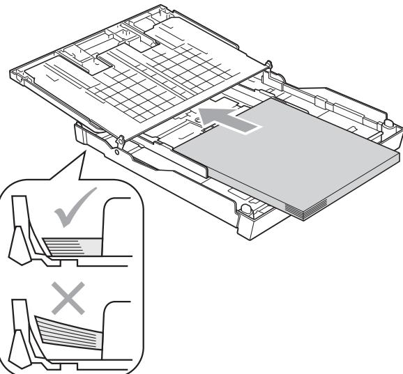
6 Gently adjust the paper side guides to the paper with both hands. Make sure the paper side guides touch the sides of the paper.
