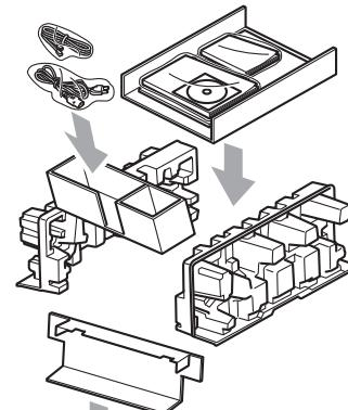
9 Pack the machine and the printed materials in the original carton with the original packing material as shown below. Do not pack the used ink cartridges in the carton.
