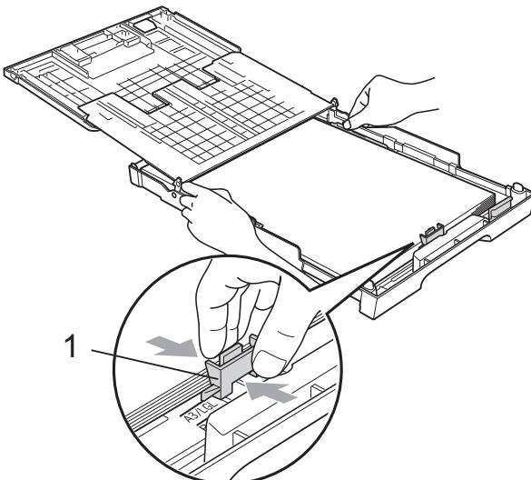
12 Close the paper tray cover and *slowly* push the paper tray into the machine. Pull out the paper support (1) until it clicks and unfold the paper support flap (2).
