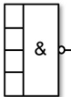
Figure 10-27 Logic gate with NAND operator
