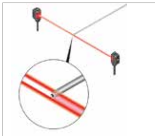
Detecting the tip of a very thin pipe
