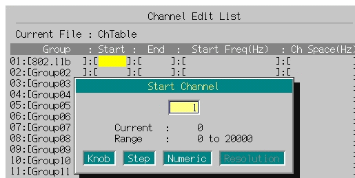
Fig. 3.3.6-3 Start channel number entry window
